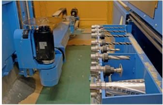
The tool changer can hold 18 tools, offering enough space for all milling, drilling and sawing tools
