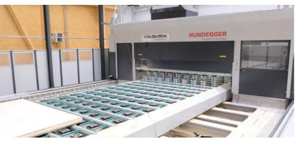
**The simultaneous infeed and discharge** of the panels saves time. The vacuum punches are lowered one row at a time during panel discharge and automatically cleaned
