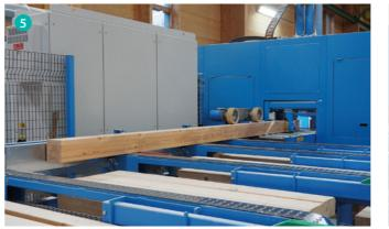
and start producing," Gerstenmayer tells us. A conveyor belt transports the sawdust and wood waste to the rear of the machine, which is also equipped with a dust extraction system.
